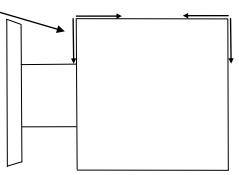
part in on the waste side of the line to the depth defined as "C1". Clear away as much wood as you can to the left of your parting line. Mark 3 more "C1" points on the surface and the free end.
