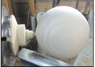
Reduce the diameter of the main spigot to get the remaining "C2" marks in, turn away the waste and sand. Part off with a thin parting tool and hand sand to a finish.
